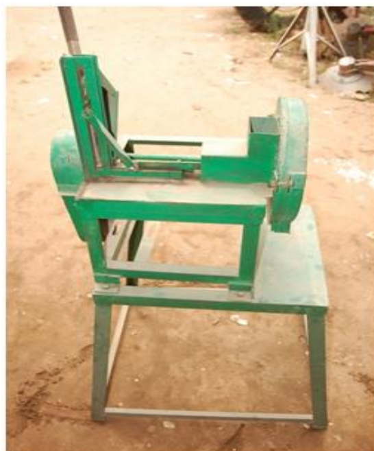
Plate 1 pictorial view of the constructed oil bean slicer
