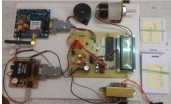
Fig.8: RFID Based security access control system with GSM technology on a single sided PCB
