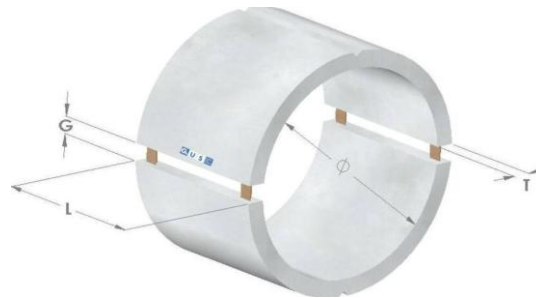
Figure 3: The bracelet square weld on anode. Source: GaUS anodes (2008).
