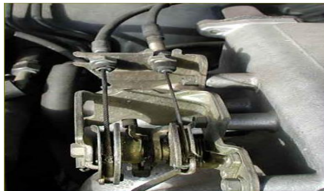
Figure 2: Cruise Control Acceleration and Deceleration [4]
