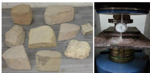
Figure 2. Testing the samples in laboratory
