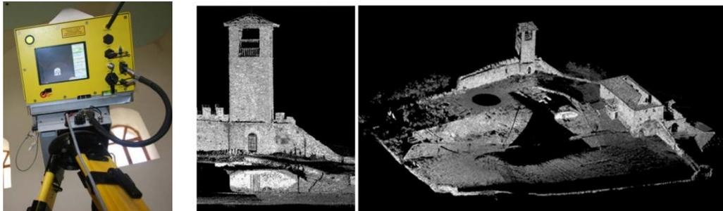
Figure 3. (a) Laser scanner used, (b) point cloud of the tower, (c) point cloud of the whole area of the castle
