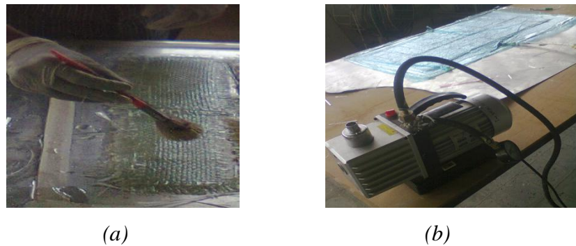
Fig. 3 Techniques of composite manufacturing used in this paper (a) Hand lay-up technique (b) HLVA technique
