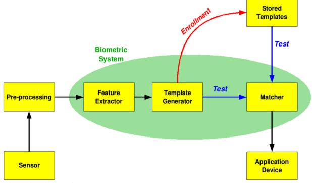
Fig.5 Working of Biometric system
