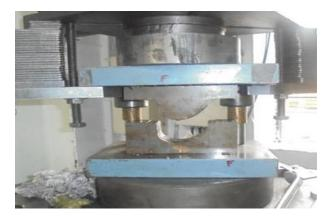
figure 7:Die Fixed in hydraulic press
