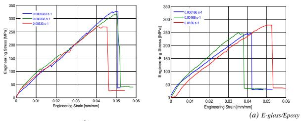
(b) E-glass/Polyester Fig. 6 Effect of Strain Rate on Tensile Strength of E-Glass/Epoxy and E-Glass/Polyester Composites
