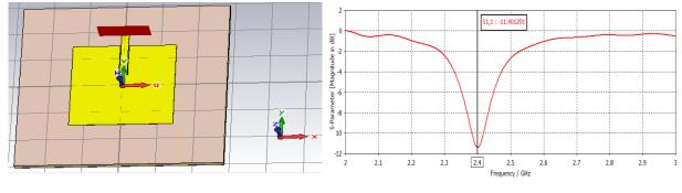
Figure 4: Designed microstrip patch antenna for FR4.
