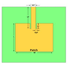
Figure 2: Parameters of microstrip patch antenna.
