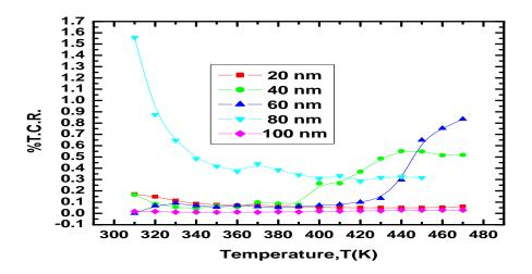
Fig-3.7: For deposited Co thin film of different thicknesses.
