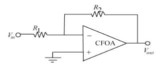
Figure 3. CFOA in inverting configuration.
