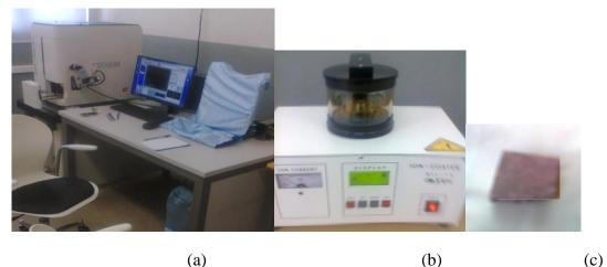
(a) (b) ( Fig. 5: (a) Scanning Electron Microscopy (b) Ion Gold Coater (c) Gold Coated Specimen
