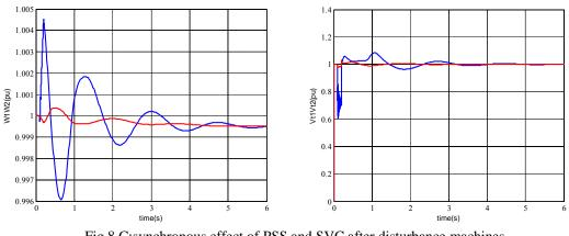
Fig 8.C:synchronous effect of PSS and SVC after disturbance, machines
