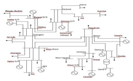
Figure 3:The 330kV, 28-bus Nigerian power system (National Control Centre, Power Holding Company of Nigeria, 2012)
