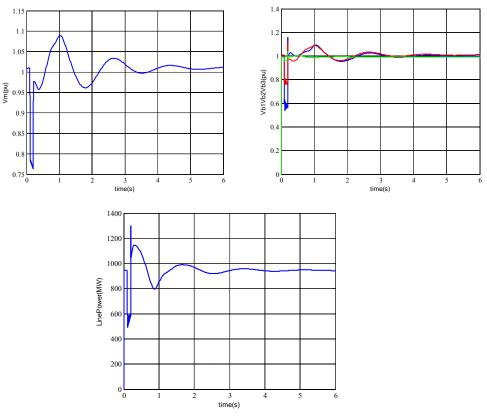
Fig 8.A:synchronous effect of PSS and SVC after disturbance,SVC compensator
