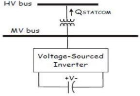
Fig 3.schematic base diagram of one STATCAM.
