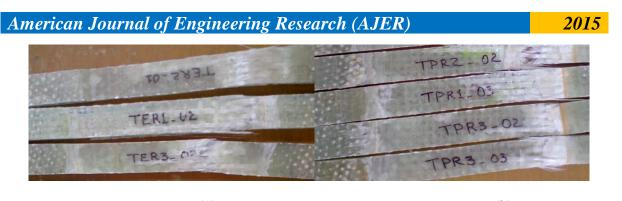
(b) (a) Fig. 7 Tensile Failure modes (a) E-glass/Epoxy composite (b) E-glass/Polyester Composite
