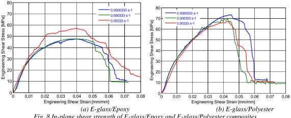
Fig. 8 In-plane shear strength of E-glass/Epoxy and E-glass/Polyester composites
