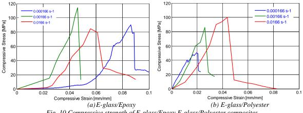
Fig. 10 Compressive strength of E-glass/Epoxy E-glass/Polyester composites
