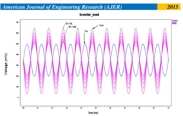
Figure 4. Response of CFOA with improved bandwidth, operating in inverting mode for different value of feedback resistor.
