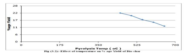
Effect of temperature on % age yield on char is again reflected in Fig 3.2. At  $450^{\circ}$ C, the maximum yield of char is obtained at  $450^{\circ}$ C.
