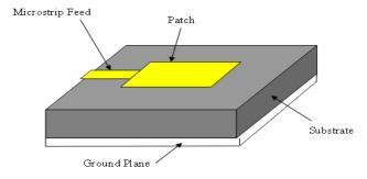
Figure 1: Structure of Patch antenna [8].
