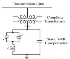
Fig 1.SVC connected to transmission line .
