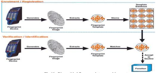
Fig.10 Bio enabled fingureprint recognition system
