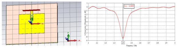
Figure 8: Designed microstrip patch antenna for RTDuroid 5880.
