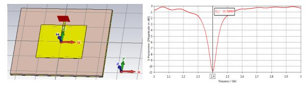
Figure 24: Designed microstrip patch antenna for Dupont-951.
