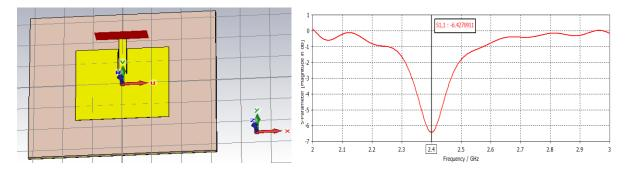
Figure 16: Designed microstrip patch antenna for Taconic.
