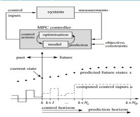
Fig. 2.3 Optimal and model predictive control
