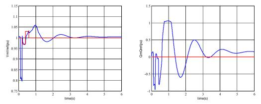
Fig 9.A:synchronous effect of PSS and STATCOM ,STATCOM compensator
