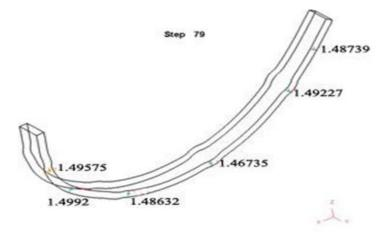
figure 6 : Variation of thickness in final component
