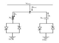
Figure1: Functional diagram of a TCR-TSC SVC
