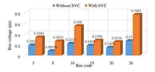
Figure 4: Weak bus voltage compensation representation
