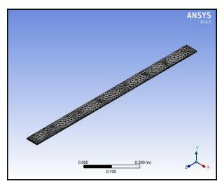
Fig. 2 : Meshing of fixed beam at one end
