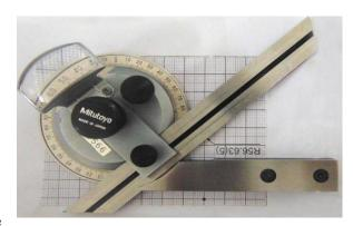
figure 10-Measurement of spring back using bevel protractor
