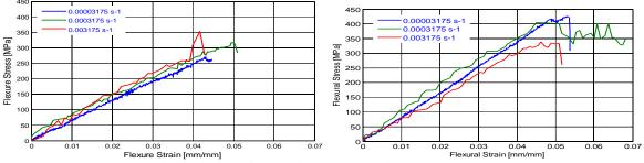
Fig. 12 Flexural strength of E-glass/Epoxy E-glass/Polyester composites
