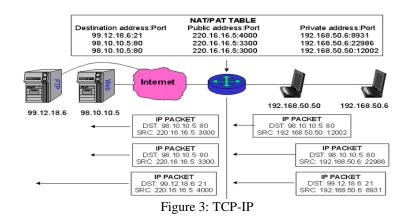
A pool of IP addresses can be shared by multiple hosts using a mechanism called Network Address Translation (NAT). NAT, described in RFC 1631, is typically implemented in hosts, proxy servers, or routers. The scheme works because every host on the user's network can be assigned an IP address from the pool of RFC 1918 private addresses; since these addresses are never seen on the Internet, this is not a problem. Consider the scenario shown in Figure 3.
