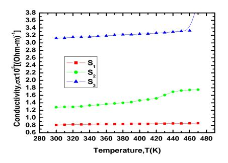
Fig-3.3: For deposited Co/TiO<sub>2</sub> multilayer thin film of different thicknesses.
