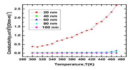
Fig-3.2: For deposited TiO<sub>2</sub> thin film of different thicknesses.
