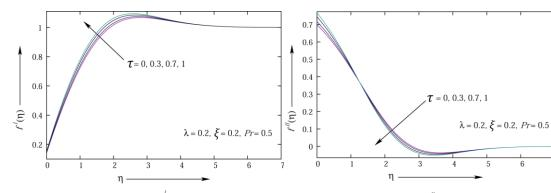
Fig. 5a Velocity profiles  $f'(\eta)$  for several values of  $\tau$
