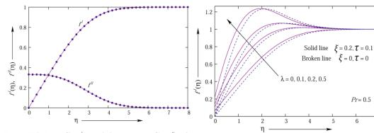
Fig. 1 Velocity profile  ${\it f}'(\eta), and shear stress profiles {\it f}''(\eta)$  for  $\lambda = 0, \ \xi = 0, \ T = 0.$
