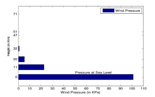
Fig. 2. Wind pressure variation with altitude
