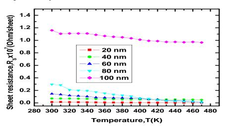
Fig-3.5: For deposited TiO<sub>2</sub> thin film of different thicknesses.
