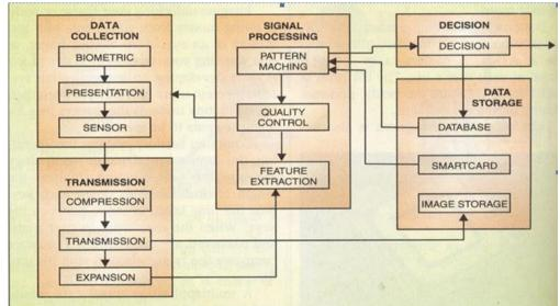
Fig. 7 Block diagram of a biometric model
