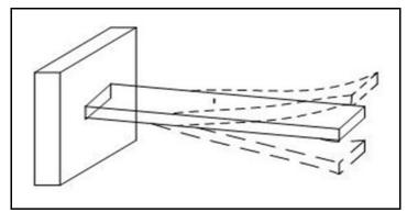
Fig. 13. Free vibration for cantilever
