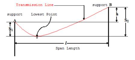
Fig.1. Formation of sag at unequal supports
