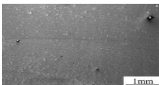
Figure 10. SEM analysis of Mild steel in 1N Phosphoric acid With HF PANI
