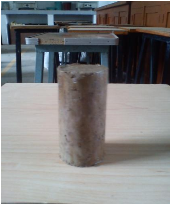
(a) Sample for UCS test (b) Author performing UCS test
