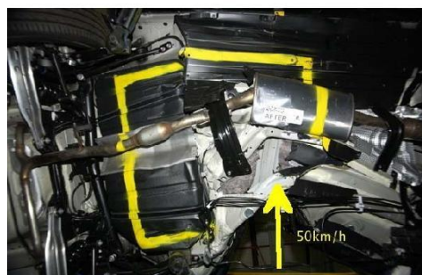
Figure 9. Underside of 50km/h vehicle. The yellow rectangle shows the approximate location of the rear floor area.
