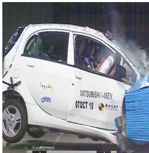
Figure 3. 64km/h offset crash test conducted by JARI for ANCAP
