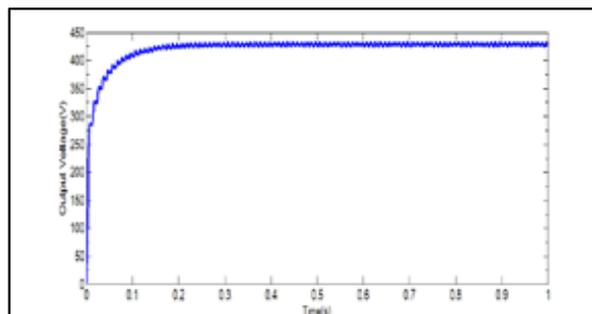
Fig. 11: Output Voltage Waveform of the Modified SEPIC
