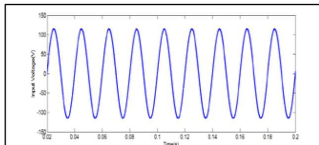
**Fig. 6: Input Voltage (115V) Waveform**
