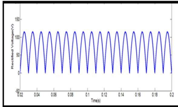
Fig. 8: Rectified Input Voltage Waveform
