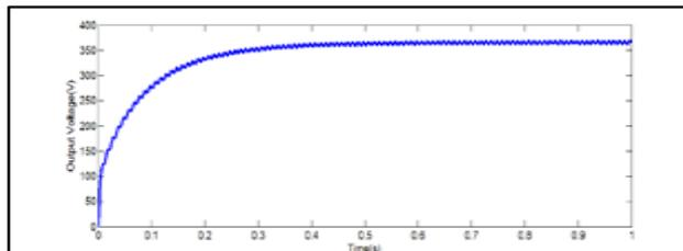
Fig. 10: Output Voltage Waveform of the Basic SEPIC
