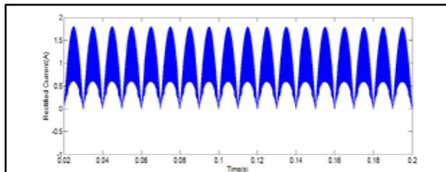
Fig. 9: Rectified Input Current Waveform
