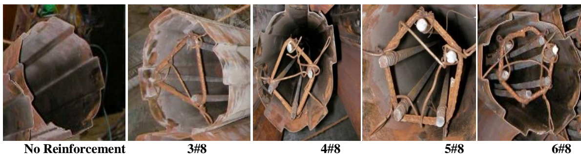
Fig 2. Rectangular Fluted Steel Tube With and Without Reinforcement
