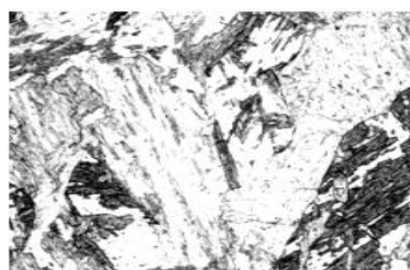
Figure 2: structural ambivalence of weld joint under post-weld heating (T = 400°C - 500°C)
