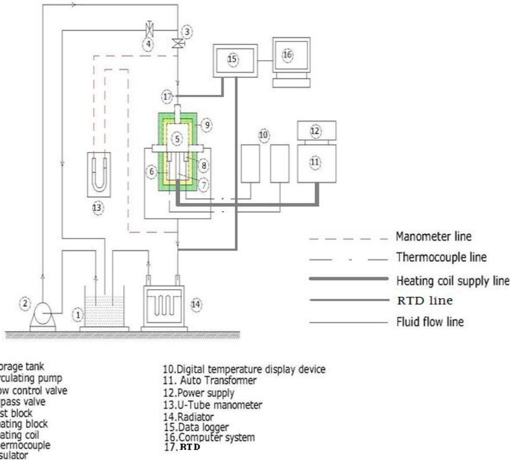
Figure.4.2. Experimental setup
