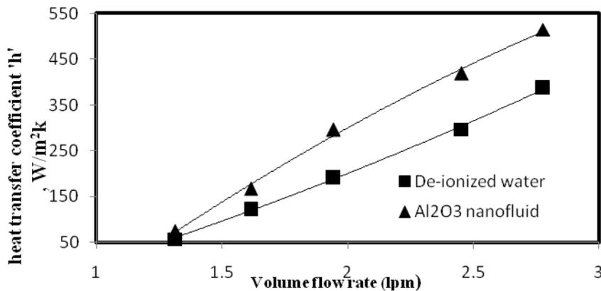
Figure.7.1. Volume flow rate  $V_s$  Heat transfer coefficient
