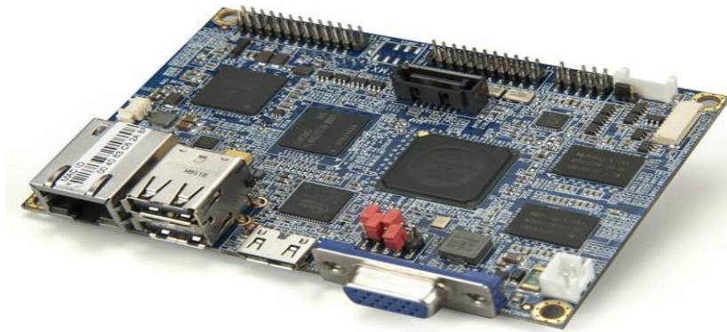
Figure 1: VIA VAB-800 10 cm x 7.2 cm Pico-ITX embedded ARM board
