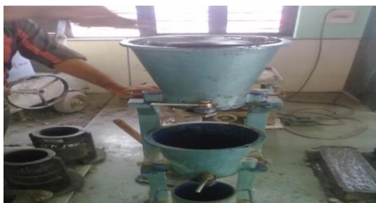
FIGURE 2. Concrete fills in upper hopper
