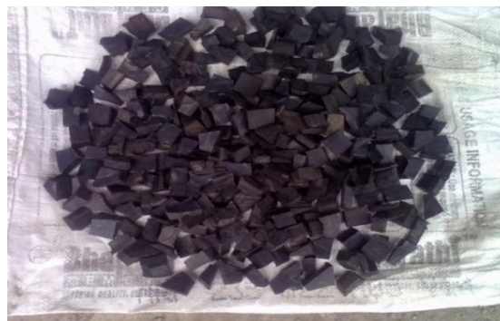
FIGURE 1. Prepared sample of chipped rubber aggregates
