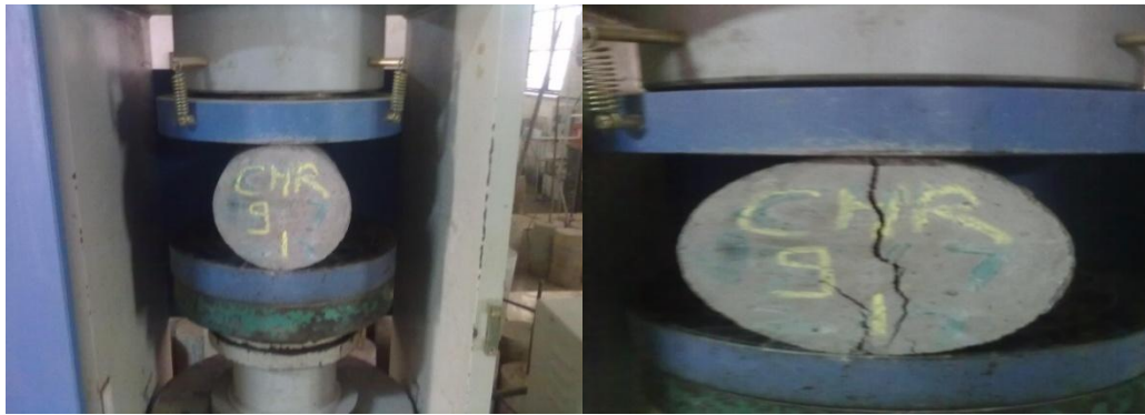
FIGURE10. Beam cylinder before failure FIGURE 11. Beam cylinder after failure
