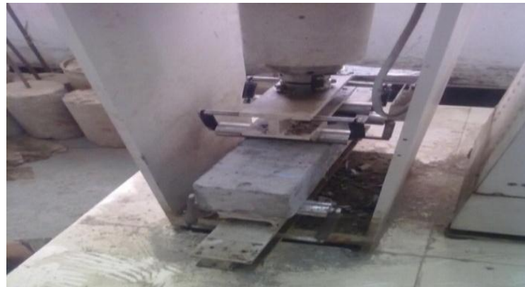
FIGURE 7. Flexural test on concrete beams
