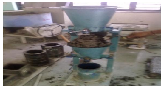
FIGURE 3. Concrete drop in lower hopper
