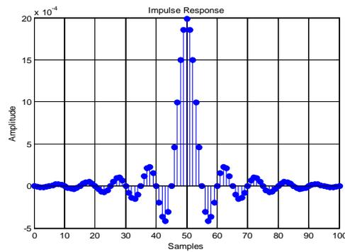
Fig 6: Impulse Response of Low Pass Filter
