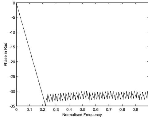
**Fig 8: Phase Response of the Low Pass Filter**
