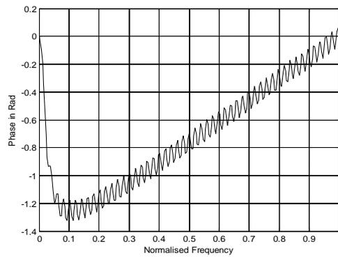
Fig 4: Phase Response of the Adaptive Filter.
