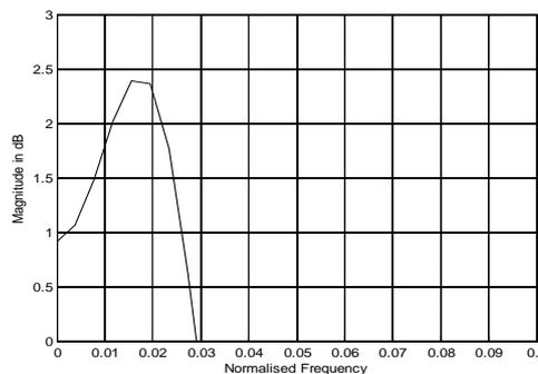
Fig 3: Magnitude Response of the Adaptive Filter
