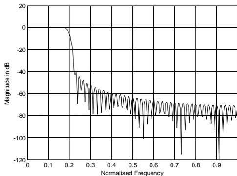
Fig 7: Magnitude Response of Low Pass Filter
