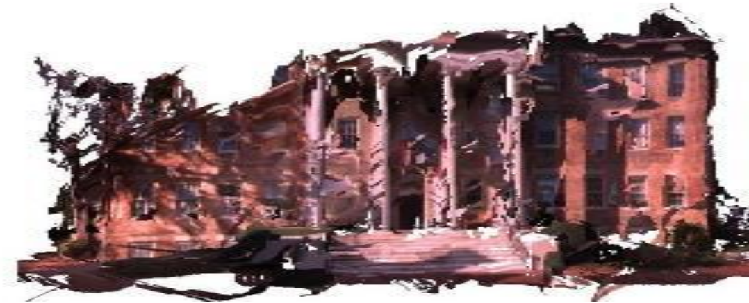
Figure1. 3D reconstruction from Video only with the back pack system (Source: [4])
