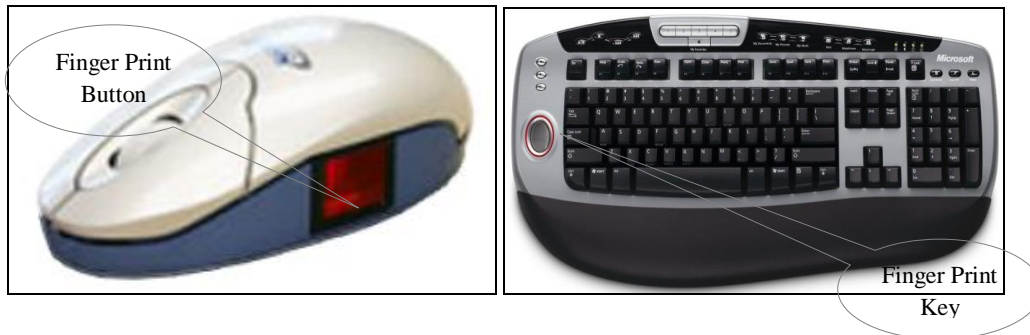
Figure 3: SecuGenOptiMousePlus Fingerprint Reader (Model MSDU03M2) and Microsoft Optical Desktop - MS BZ5-00002
