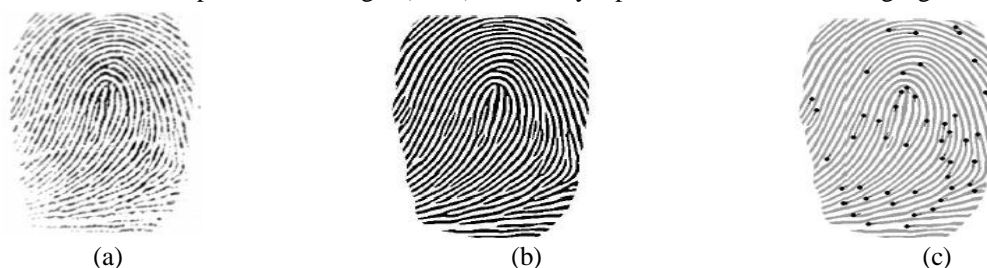
Figure 1: Feature Extraction Process: (a) Original Image (b) After Edge Detection, (c) Including Feature Points
