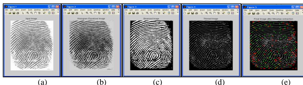
Figure 2: (a) Original Image (b) Gray Scale Image (c) Binarized Image (d) Thinned Image (e) Final Minutiae
