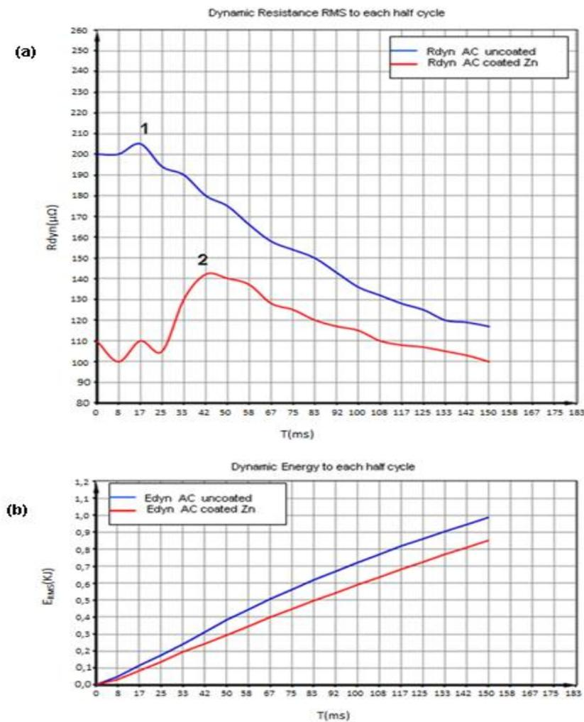
Figure 10 - (a) RMS dynamic resistances ( $\mu\Omega$ ) and (b) RMS dynamic energies (kJ) in AC welding in zinc coated and uncoated steel sheets, as a function of time (ms).
