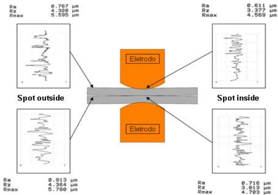
Figure 12 - Example of surface roughness of steel sheets inside and outside of the action line of the force exerted by the electrodes, with a force of 260 kgf.
