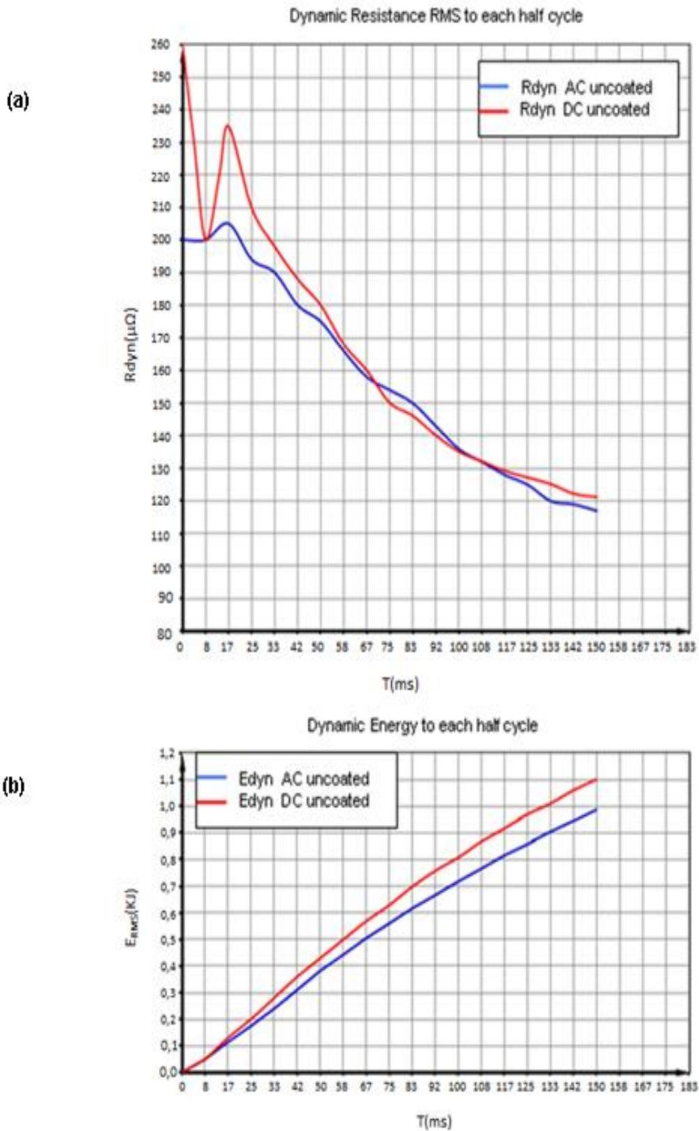
Figure 7 – (a) RMS dynamic resistances ( $\mu\Omega$ ) and (b) RMS dynamic energies (kJ) in AC and DC welding in uncoated steel sheets, as a function of time (ms).
