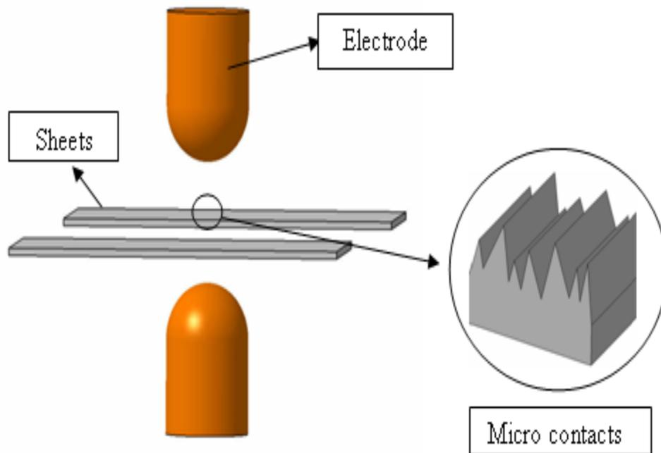
Figure 2 - Sheet surface roughness which defines the contact resistance.
