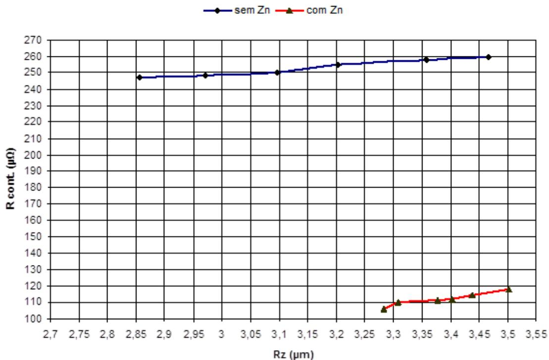
Figure 13 - Contact electrical resistance ( $R_{cont.}$   $\mu\Omega$ ) versus surface roughness ( $R_z$ - $\mu m$ ) inside the spot in Zn coated and uncoated sheets using an electrode force of 260kgf.
