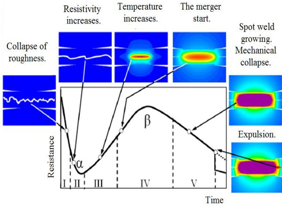
Figure 3 - Scheme of the dynamic electrical resistance during the formation of a nugget. Adapted from reference [11].
