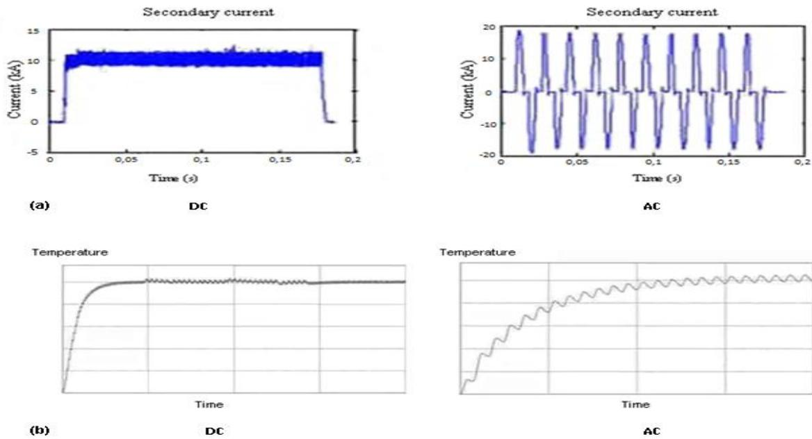
Figure 4. (a) Shape of the DC and AC current outputs [12]; (b) Heat generation in DC and AC welding equipments [8].
