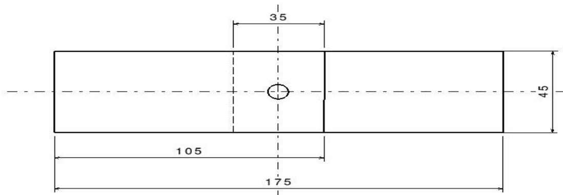
Figure 5- Dimensions of specimen in accordance to standard EN ISO 14273.
