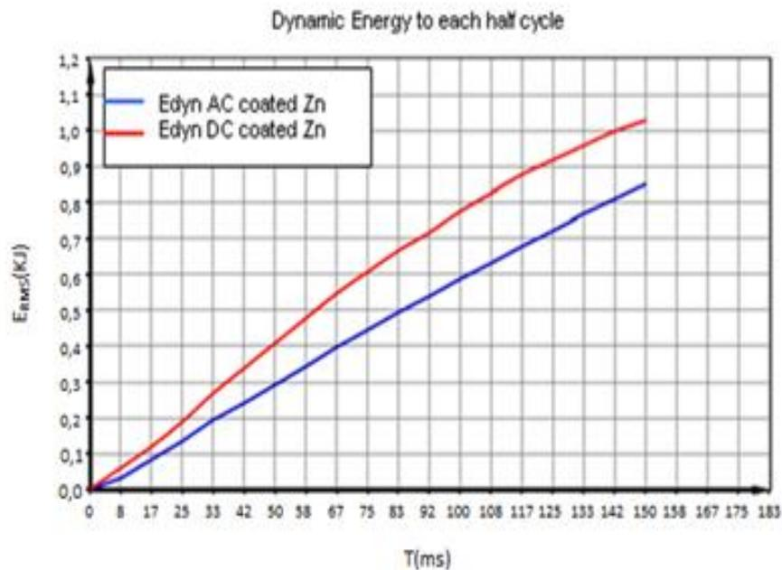
Figure 8 – (a) RMS dynamic resistances ( $\mu\Omega$ ) and (b) RMS dynamic energies (kJ) in AC and DC welding in zinc coated steel sheets, as a function of time (ms).
