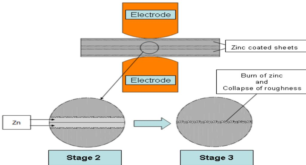
Figure 9 - Schematic drawing of the zinc burn (melting, vaporization and diffusion) represented by stages 2 and 3 of figure 8(a).
