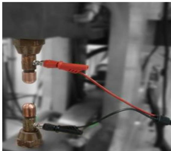
Figure 6 - Differential probe tip to measure the voltage during welding.
