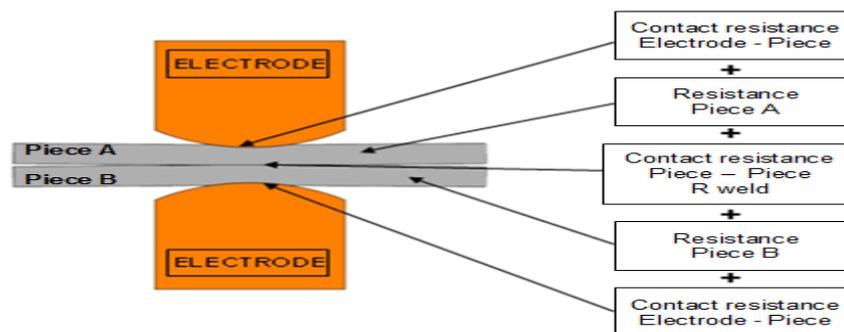
Figure 1- Scheme of electrical resistance between the electrodes in resistance spot welding.
