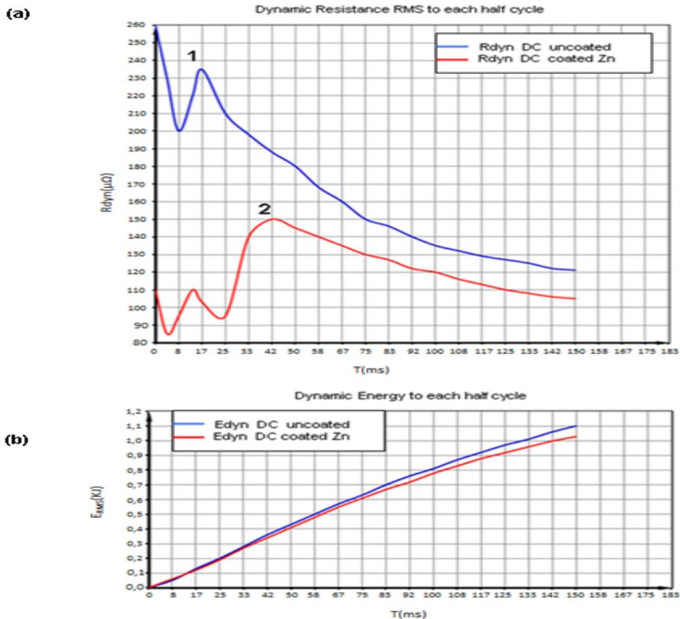
Figure 11 - (a) RMS dynamic resistances ( $\mu\Omega$ ) and (b) RMS dynamic energies (kJ) in DC welding in zinc coated and uncoated steel sheets, as a function of time (ms).
