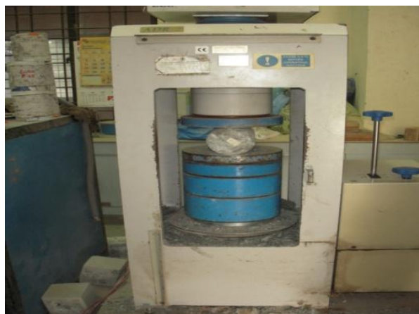
Plate No3 Test Set up for measuring Split Tensile Strength
