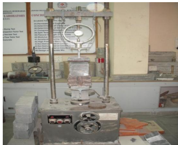
Plate No2 Test Set up for measuring Flexural Strength
