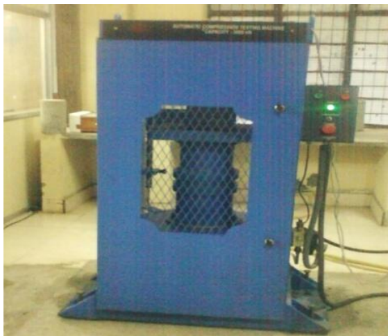
Plate No1 Test Set up for measuring Compressive Strength
