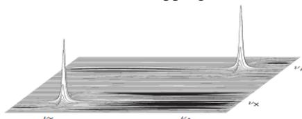
**Figure-1:** Sample containing two uncoupled spins, A and X, of offsets  $\nu_A$  and  $\nu_X$ . Each produces a 2D peak at its corresponding chemical shift offset in both dimensions.
