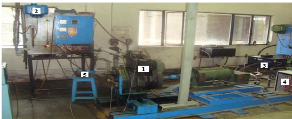
1 - Kirloskar Vertical C.I. Diesel Engine, 2 - Fuel Tank, 3 – AVL 437 C Smoke meter, 4 – Electrical loading device, 5 – Engine temperature monitor
