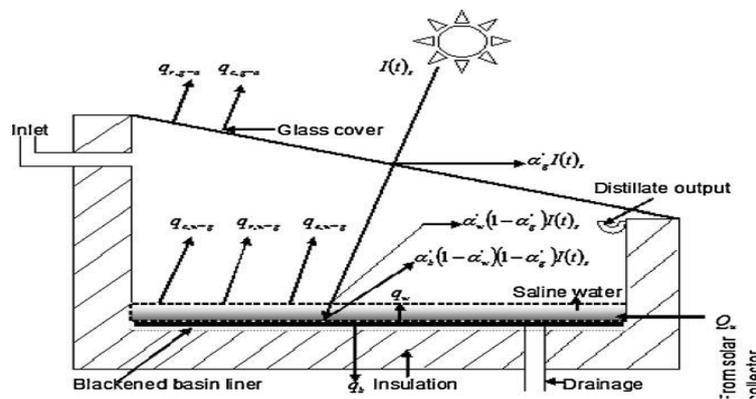
Figure 2: Energy flow diagram of single slope solar still.
