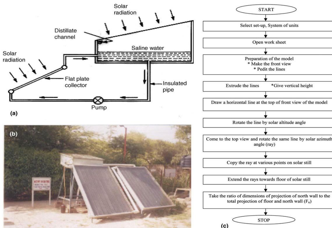
Figure 3 (a): Schematic diagram of an active solar still coupled with a flat plate collector, (b) photograph of the experimental set-up and (c) flow chart of the AUTOCAD 2000 model.
