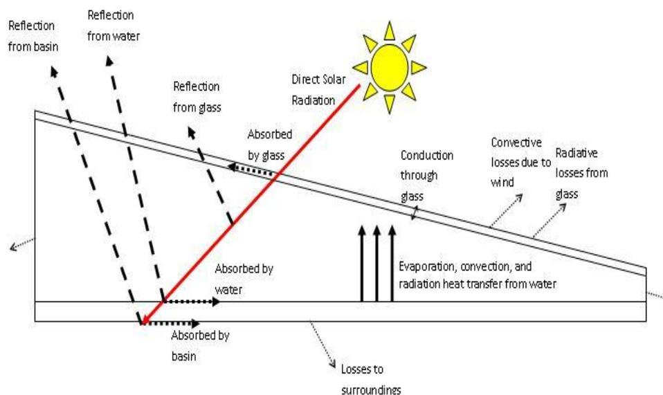
Figure 1: Simple solar water distillation process
