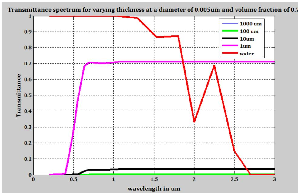
**Fig 2:** Transmittance spectrum of hematite nanofluid at different thicknesses of liquid layer. Basefluid transmittance (in red) is at l=1000µm.
