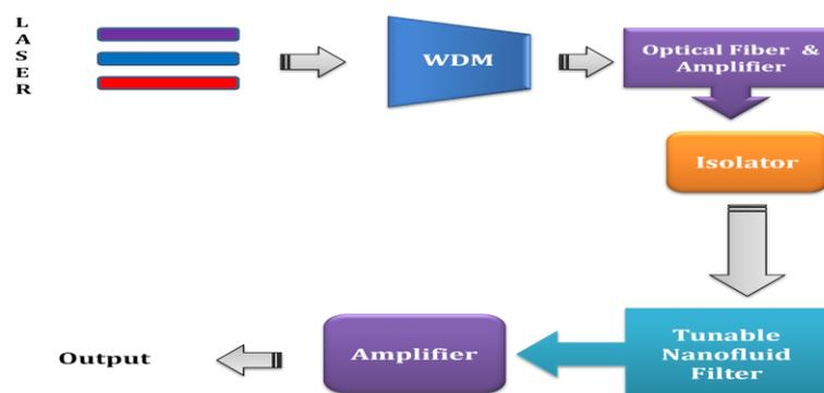
Fig 1: Block diagram of a tunable Nanofluid Filter application in a transmitter circuit.
