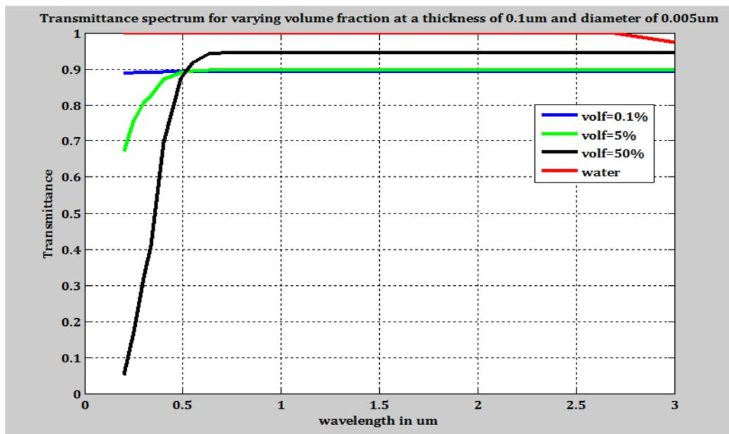
Fig 4: Transmittance spectrum for varying volume fraction of hematite nanofluid.
