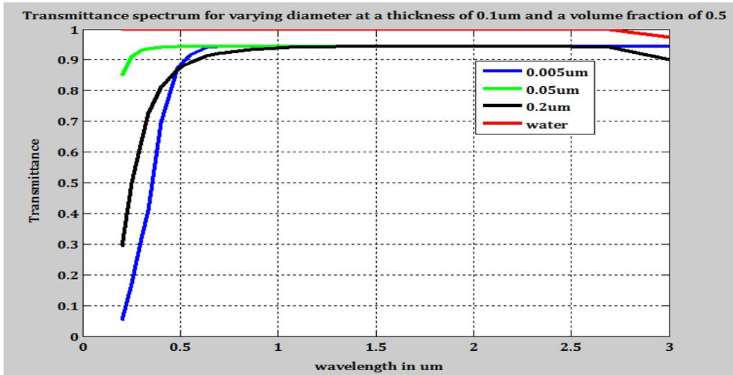
Fig 3: Transmittance spectrum of hematite nanofluid at different particle diameters.
