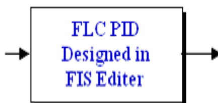
Fig.4 Masked subsystem of Fuzzy Logic PID Controller designed in MATLAB
