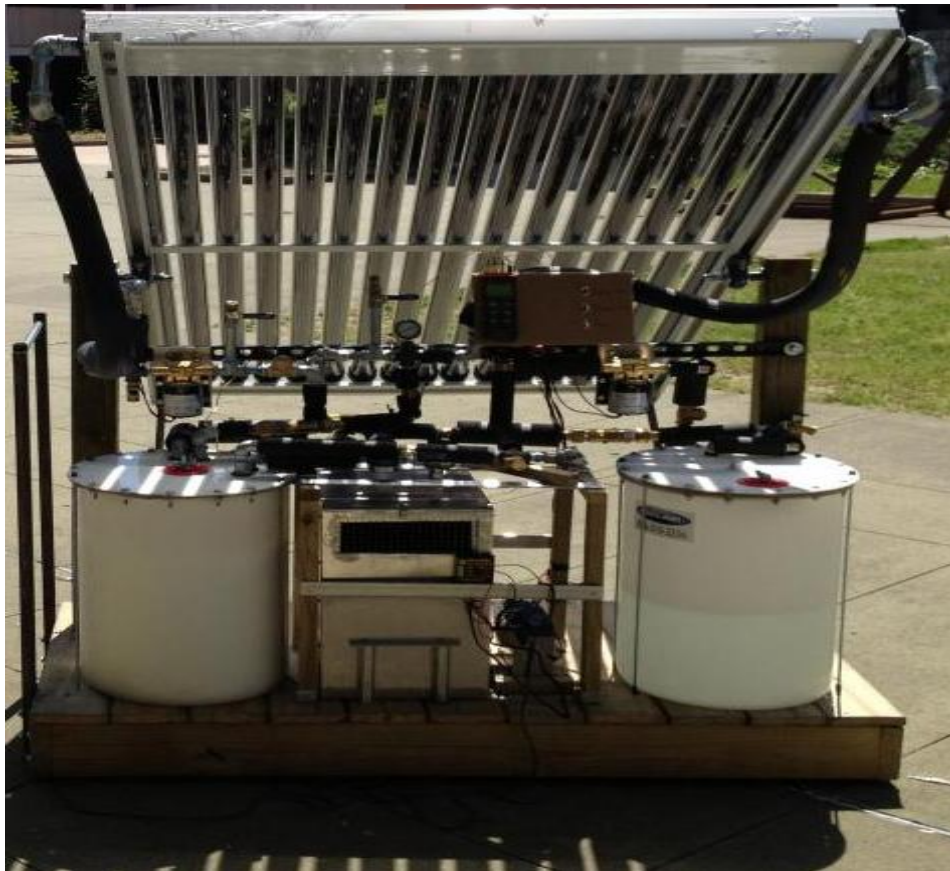
Figure 1. System setup (View from the back of the Solar Collector)
