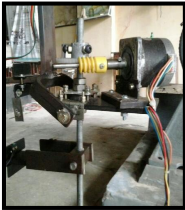
Fig 7. Gear Mechanism for Hybrid Axis
