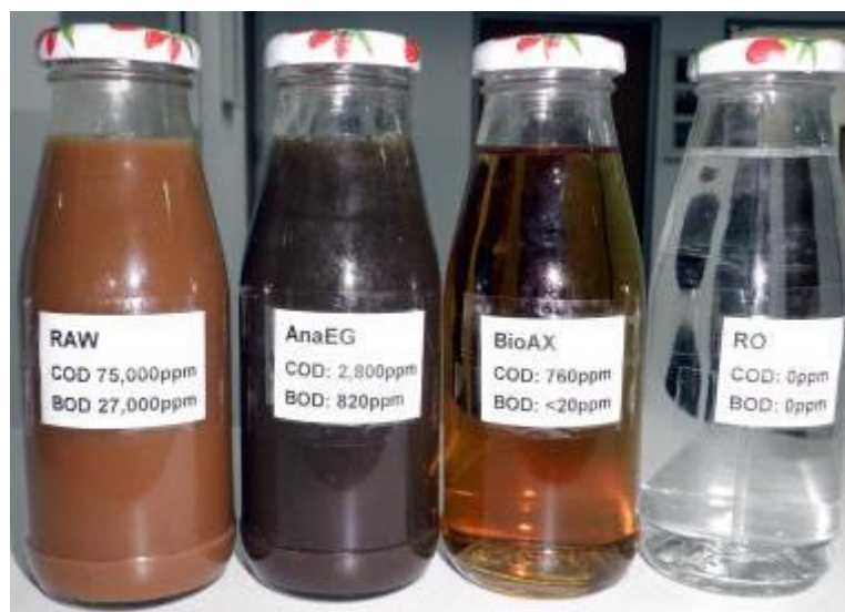
Figure1. Pilot project of Ronser Bio-Tech's Zero Discharge POME treatment technology at Labu, Negri Sembilan
