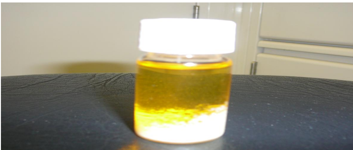
Figure 3: PETE and HDPE waste plastics mixture to fuel with wax
