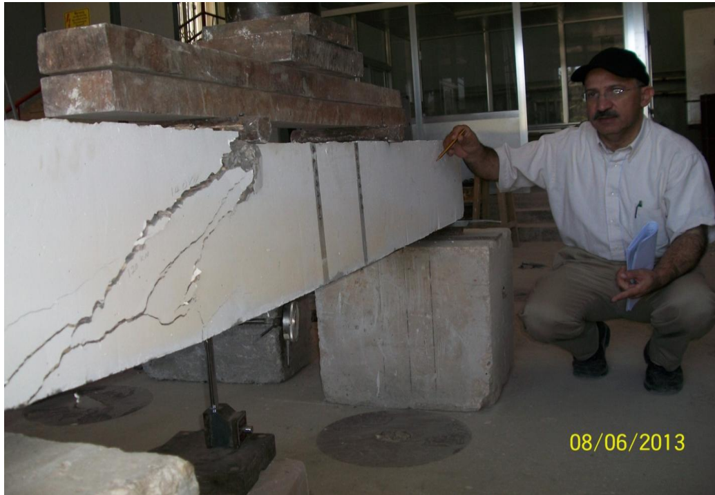
Figure 6: Beam BU at failure stage
