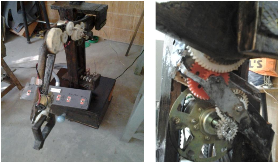
Fig. 9 increasing torque by adding external gear
