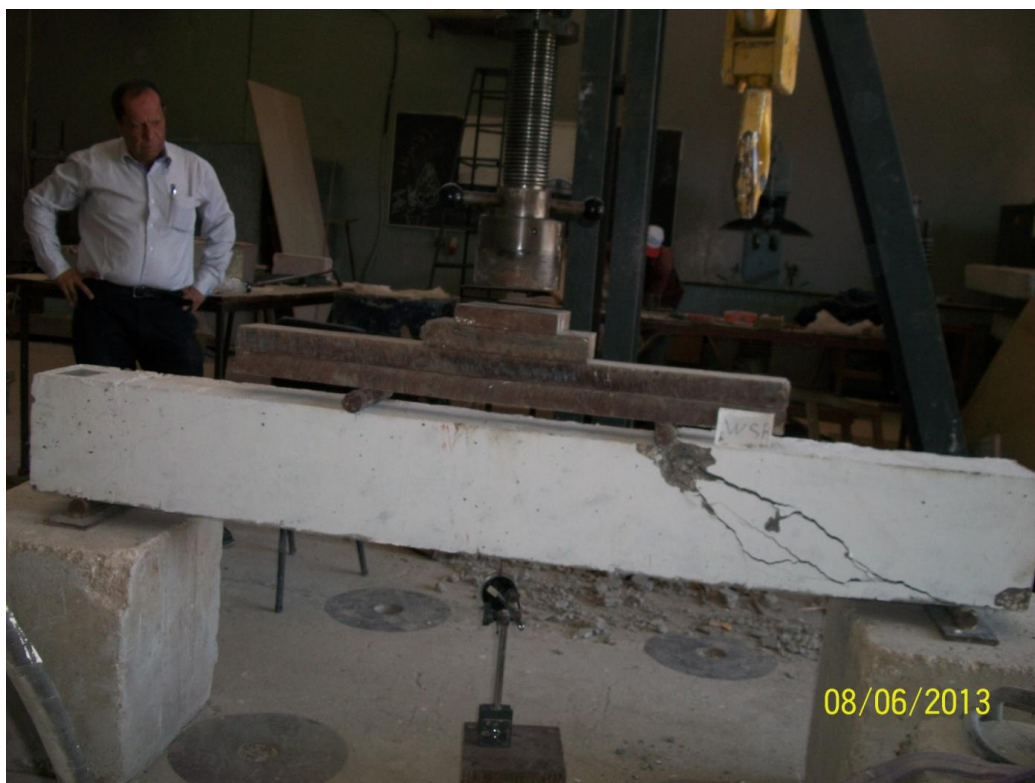
Figure 7: The mode of failure of the welded beam BW.
