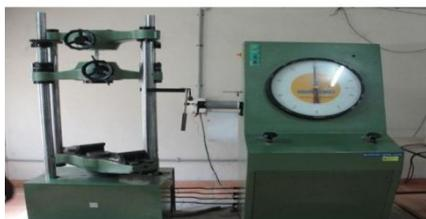
Fig 2: Universal Testing machine
