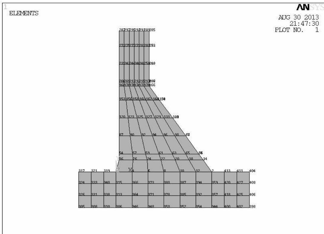
Fig.3 Finite Element Mesh of Perunthenaruvi Dam
