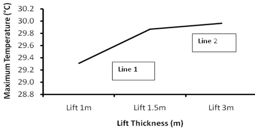
Fig.5 Maximum temperature Vs Lift Thickness
