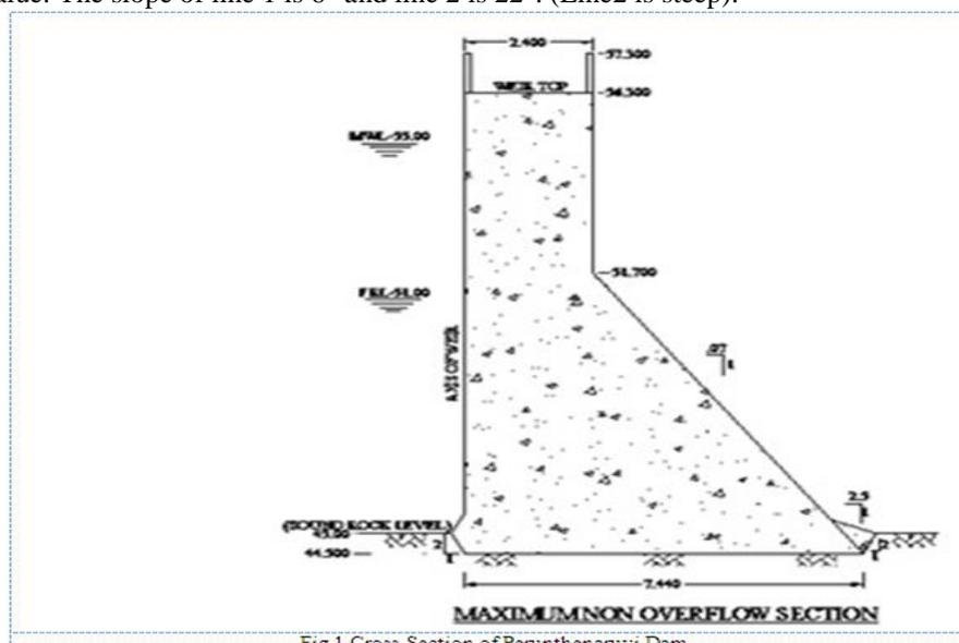
Fig.1 Cross Section of Perunthenaruvi Dam
