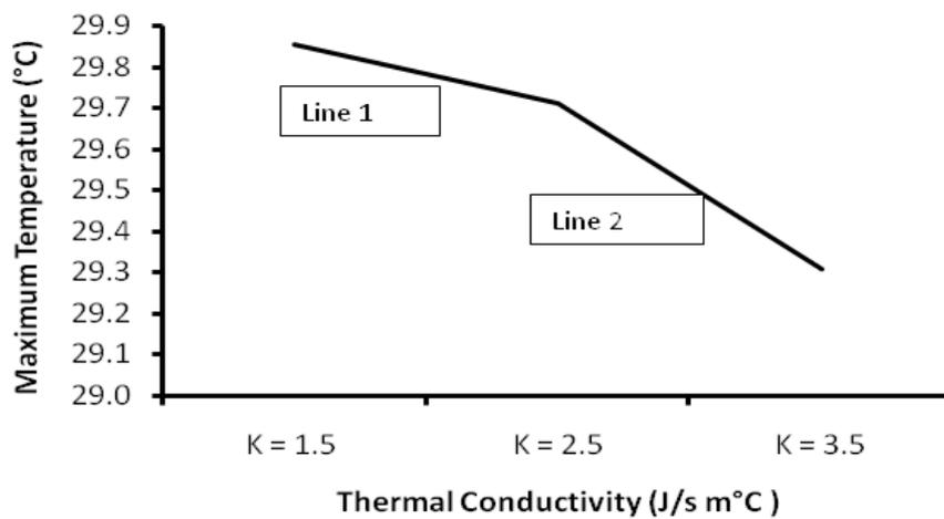
Fig.6 Maximum temperature Vs Thermal Conductivity
