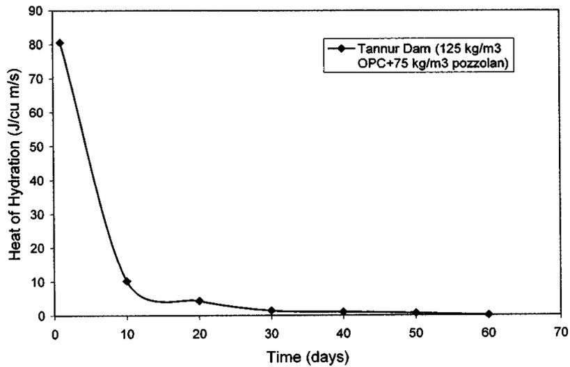
Fig.2 Heat of Hydration
