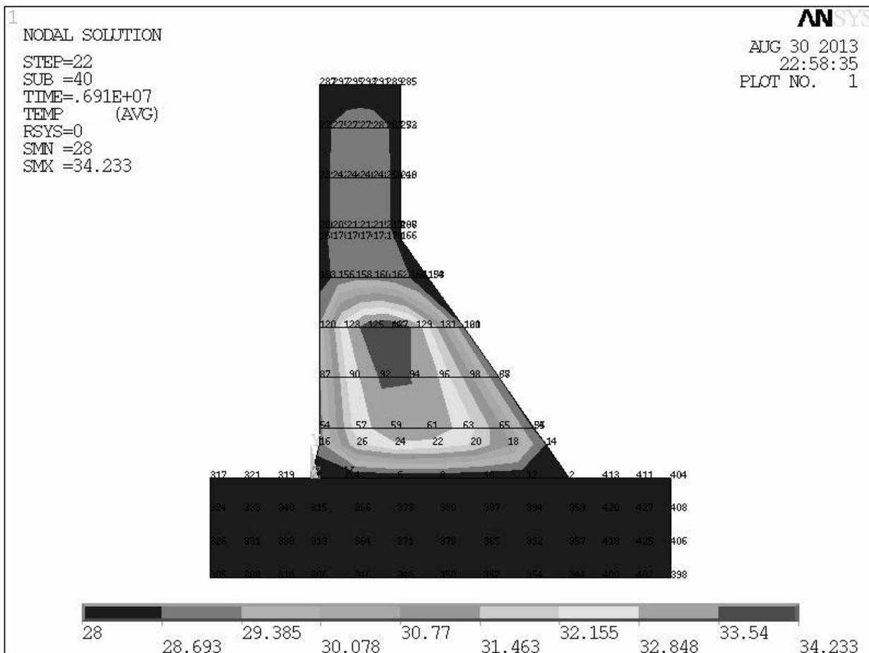
Fig.8 Temperature distribution for C=950 J/kg °C, IT=25 °C, Lift =1.5m and k= 3.5 J/s m °C
