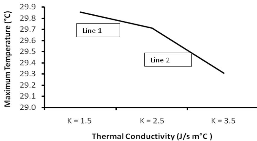
Fig.6 Maximum temperature Vs Thermal Conductivity
