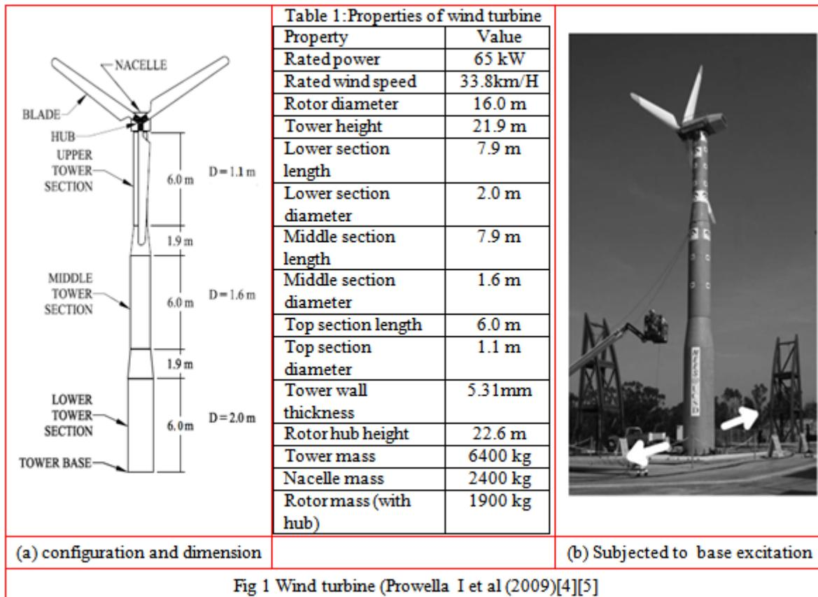
Excitation used for the tests was derived from a recording of the Desert Hot Springs (DHS) East-West component of the June 28th, 1992 Landers Earthquake (Prowella I et al (2009)[4][5] .DHS is a California Strong Motion Instrumentation Program (CSMIP) station situated on deep alluvium located 23 km from the fault trace where the Landers Earthquake occurred. The fig 1(c) shows the turbine subjected to base excitations in the east-west direction.
