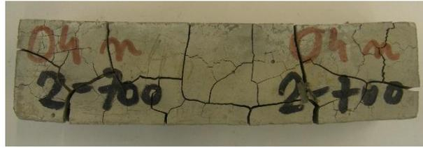
Fig. 3. A sample of paste w/c = 0,4 after heating in an furnace at 700°C.
