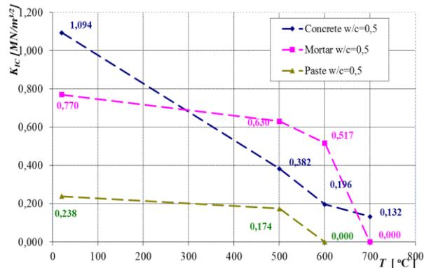
Fig. 5. Relationships of  $K_{IC}$  - T of concrete, paste and mortar for w/c = 0,5 under the influence of fire temperatures.
