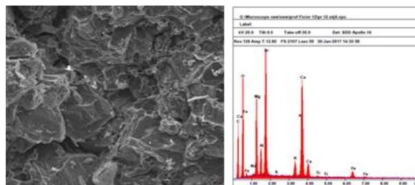
**Fig. 7. Sample SEM photo and EDS microanalysis of concrete for w/c = 0.4 after exposure to fire temperatures.**
