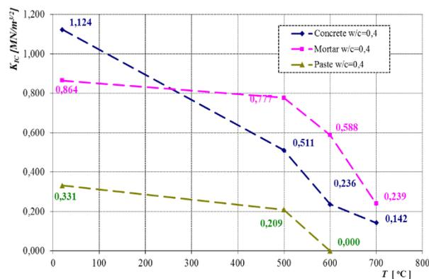
Fig. 4. Relationships between  $K_{IC}$  -  $T$  of concrete, paste and mortar for  $w/c = 0,4$  under the influence of fire temperatures.
