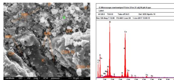
**Fig. 8. Sample SEM photo and EDS analysis of mortar for w/c = 0.4 after exposure to fire temperatures: CH - portlandite, CSH phase, MR - micro-cracks, P - pores, K - aggregate.**
