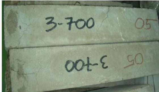
**Fig. 1. Concrete sample for  $w/c = 0,5$  after application of fire temperature  $700^{\circ}\text{C}$ .**
