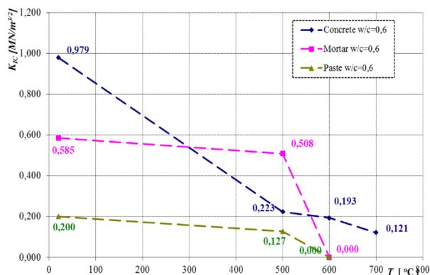
Fig. 6. Relationships between  $K_{IC}$  - T of concrete, paste and mortar for w/c = 0,6 under the influence of fire temperatures.
