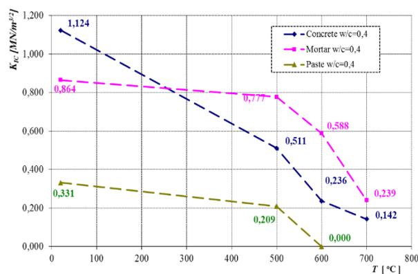
Fig. 4. Relationships between  $K_{IC}$  -  $T$  of concrete, paste and mortar for w/c = 0,4 under the influence of fire temperatures.
