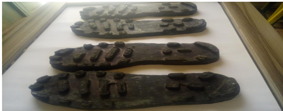
Plate 9: Produced combat boot sole prototypes showing studs
