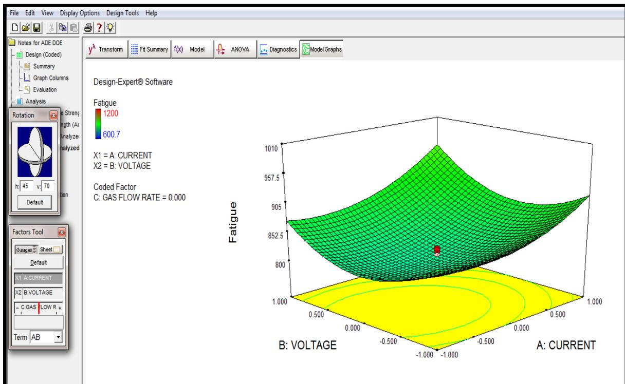
Figure 3.2: A surface plot of voltage and current on fatigue
