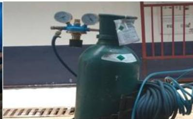
Figure 2.2: TIG Shielding Gas Cylinder
