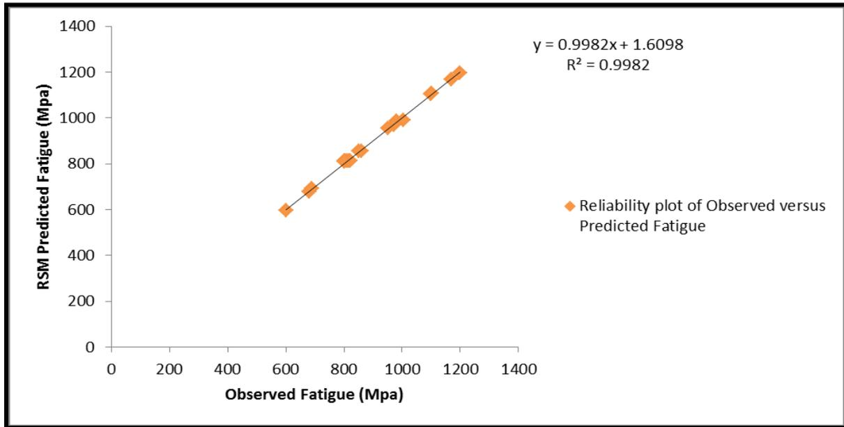
Figure 3.1: Reliability plot of observed versus predicted fatigue
