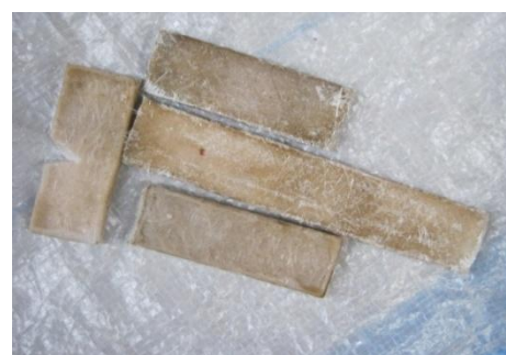
Plate III: Some samples of reinforced MKO resin test specimens
