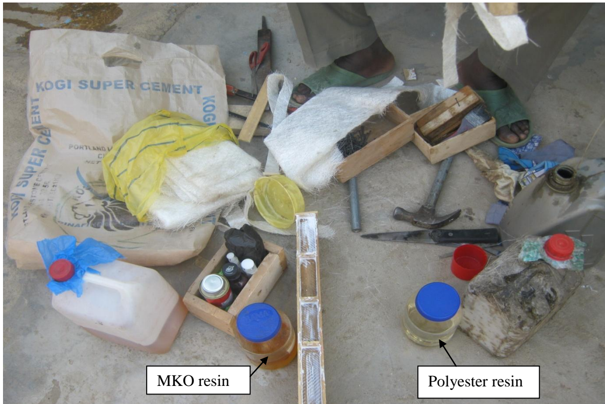
Plate I: Materials for production of specimens from both MKO and Polyester resins.
