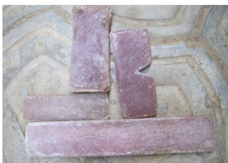
Plate II: Some sample of reinforced polyester resin test specimens
