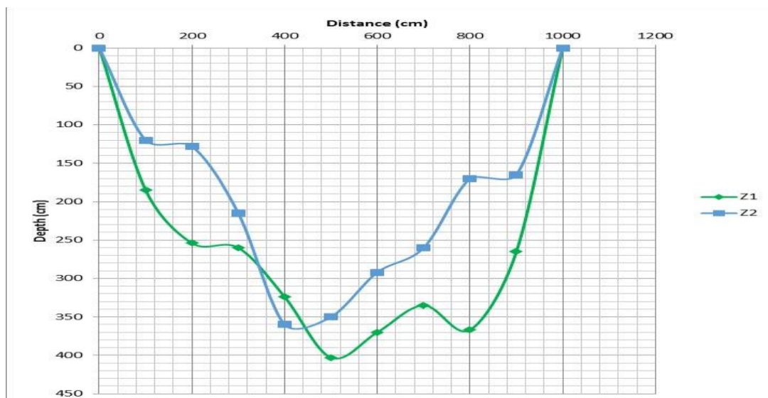
Figure1: Scale Picture of a Slice through River Asa at Z 1 and Z 2 in September, 2018
