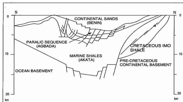
**Figure 1:** Axial Portion of Niger Delta Showing the Relationships of the Tripartite Division of the Tertiary Sequence to Basement (Doust and Omatsola, 1990).
