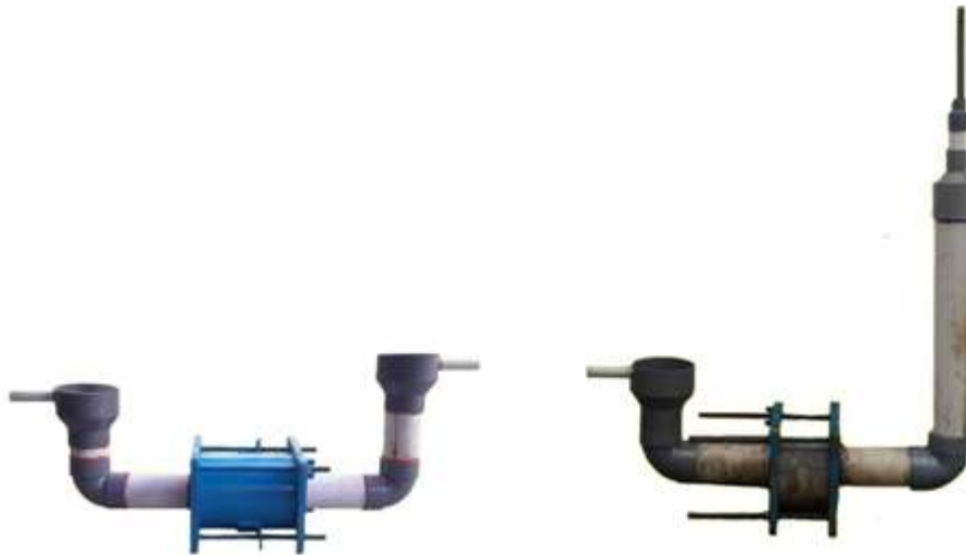
Figure 3. Fabrication equipment of Horizontal permeability. Left: Constant Head. Right: Falling head
