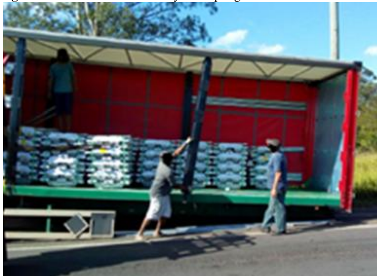
Figure 4 - Loss due to involuntary decoupling of the Sider slide assembly
