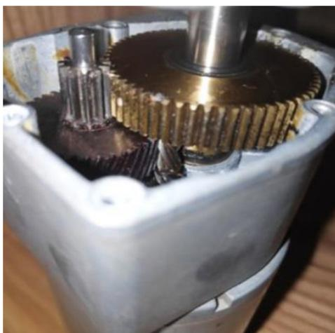
Fig. 5. Two stages gearbox with 44.73 reduction ratio
