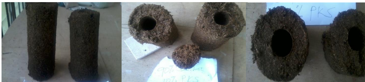
Figure 3: Samples of the Produced Composite Biomass Briquettes
