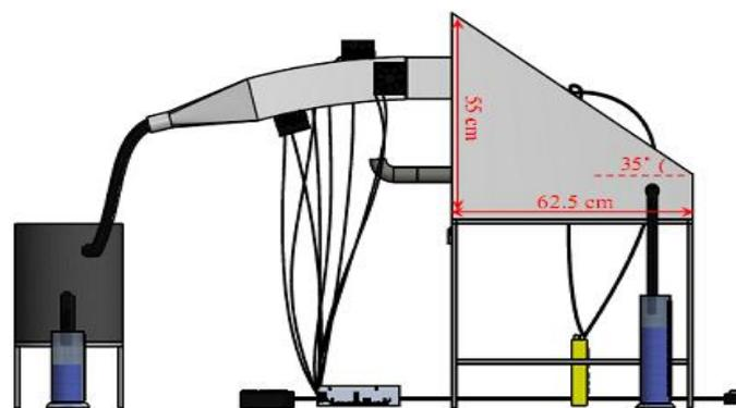
Fig.24: Schematic of the modified solar still [67].
