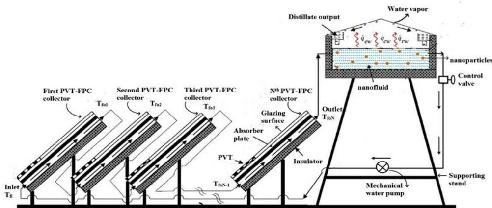
Fig. 22: Active solar still with no and with internal heat exchanger [65].
