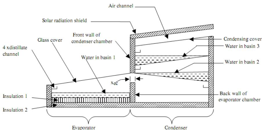
Fig.14: Schematic of separate condenser with passive solar still [55].
