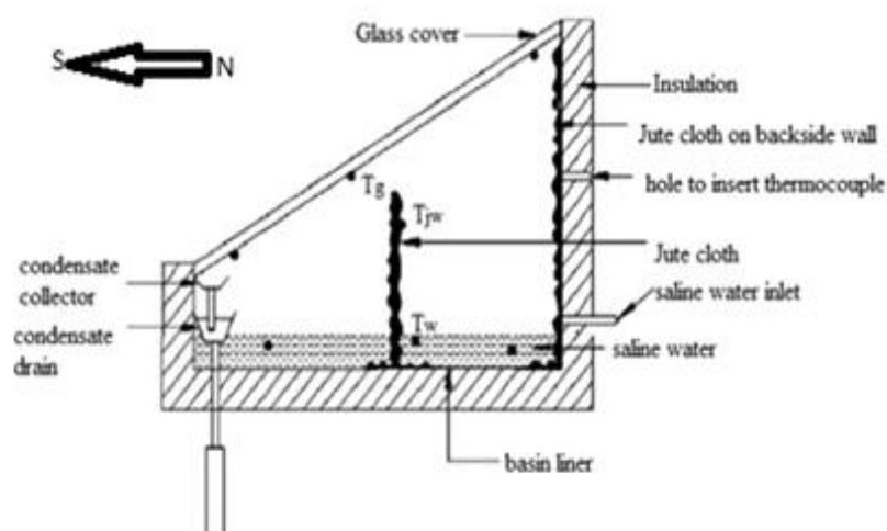
Fig.2: Schematic diagram of jute cloth solar still [14].
