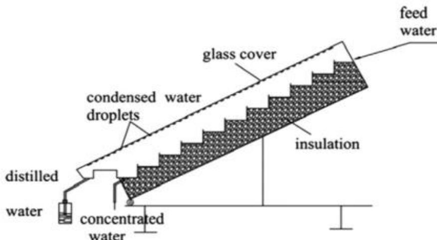
Fig.10: Weir cascade solar still [46].
