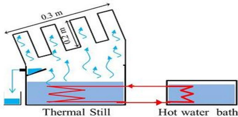
Fig. 21: Schematic of modified still [64].
