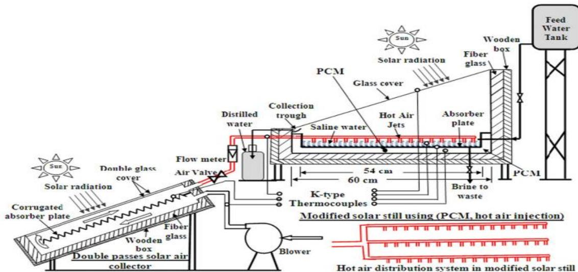
Fig. 18: Schematic of the modified system [60].
