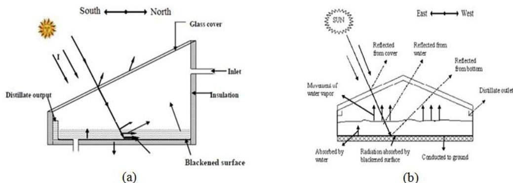
Fig. 1: (a)-Single slope solar still (b)-Double slope passive solar still [11].
