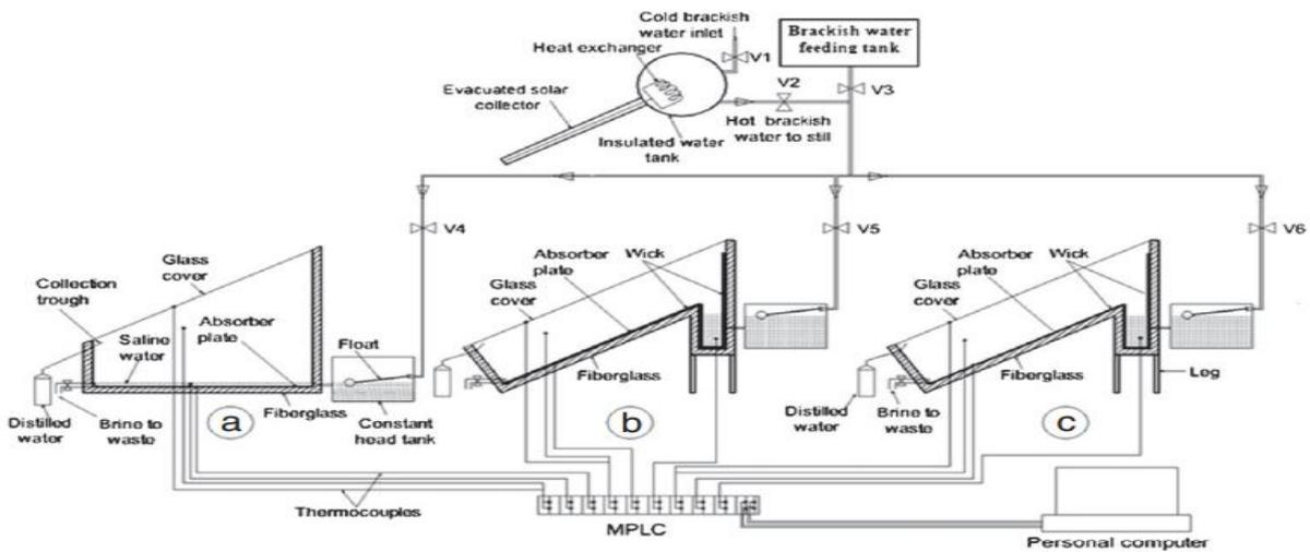
Fig. 13: Schematic of (a) Conventional still. (b) Double layer wick still. (c) Single wick solar still [54].
