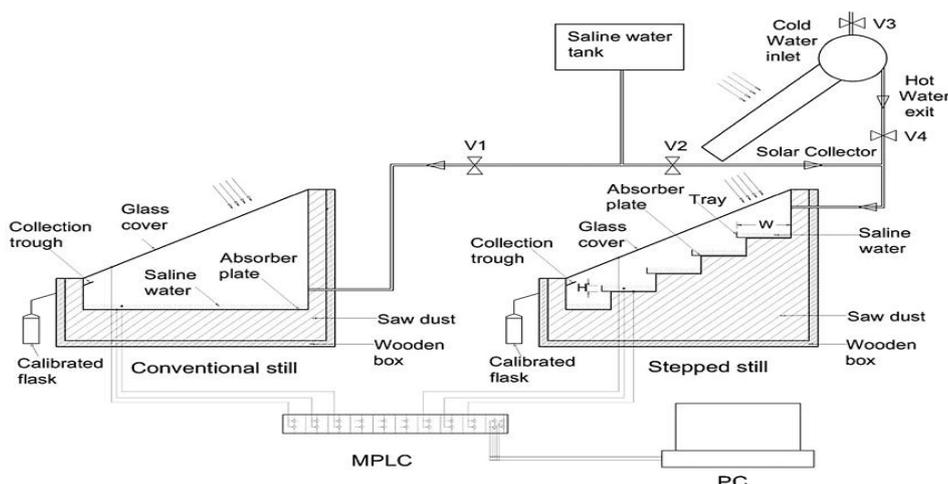
Fig.16: Schematic of the experimental set up [58].
