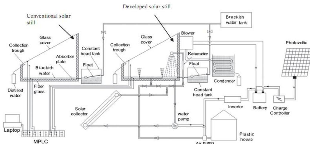
Fig.15: Schematic of the experimental set up [57].
