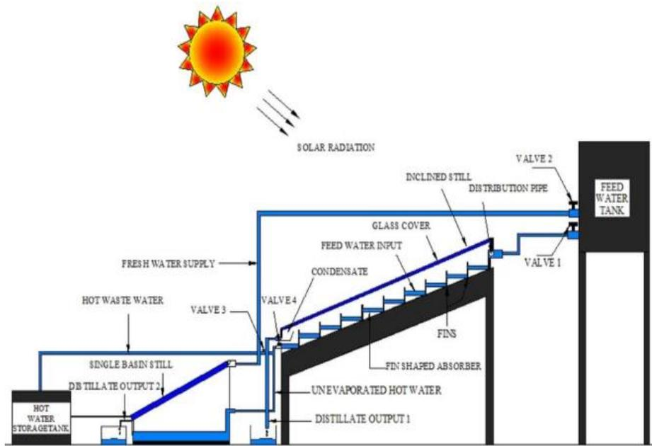
Fig.12: Schematic of integrated desalination system [51].
