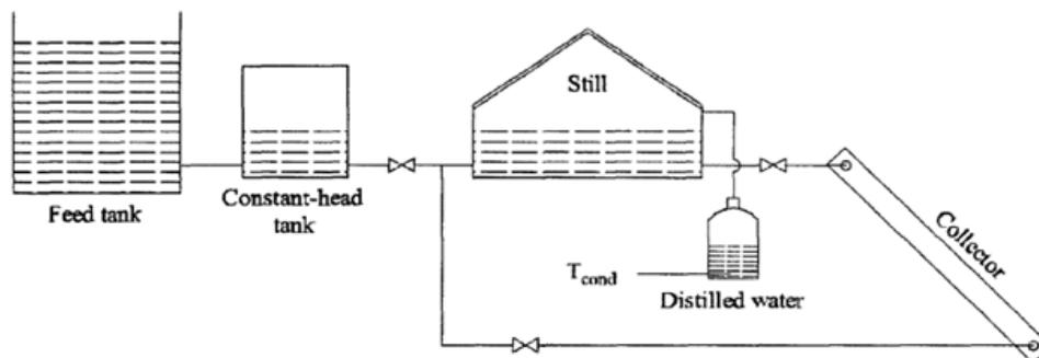
Figure 8: Schematic of test rig [39].
