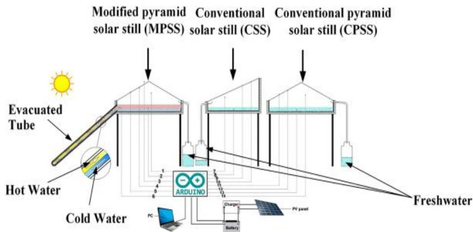
Fig.23: Schematic of the experimental setup [66].
