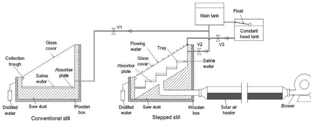
Fig.7: Schematic of test rig [38].
