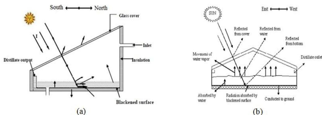
Fig. 1: (a)-Single slope solar still (b)-Double slope passive solar still [11].
