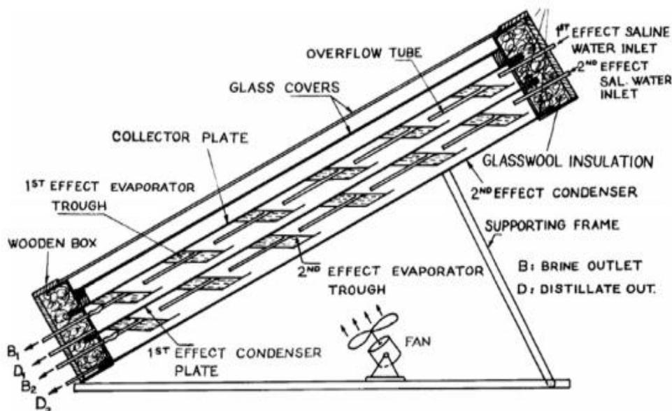
Fig.5: Schematic of tilted multi-effect solar still [28].
