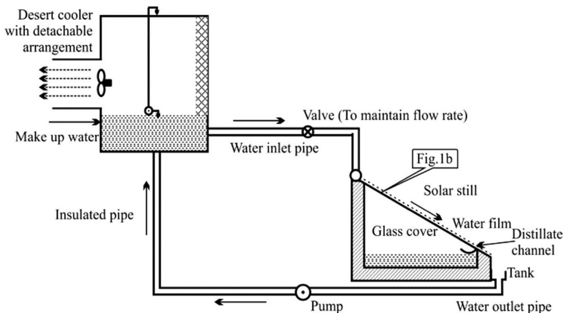
Fig. 20: Schematic of the system [63].
