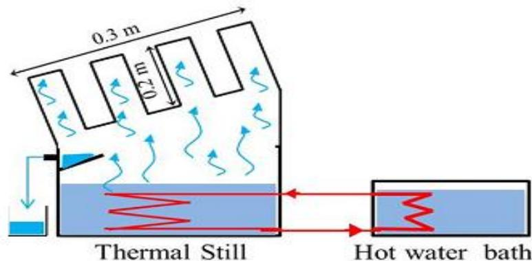
Fig. 21: Schematic of modified still [64].
