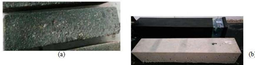
**Fig. 2** Appearance of AASC specimens after 300 freeze-thaw cycles. (a) Specimens with NaOH as activator;(b) Specimens with water glass as activator.
