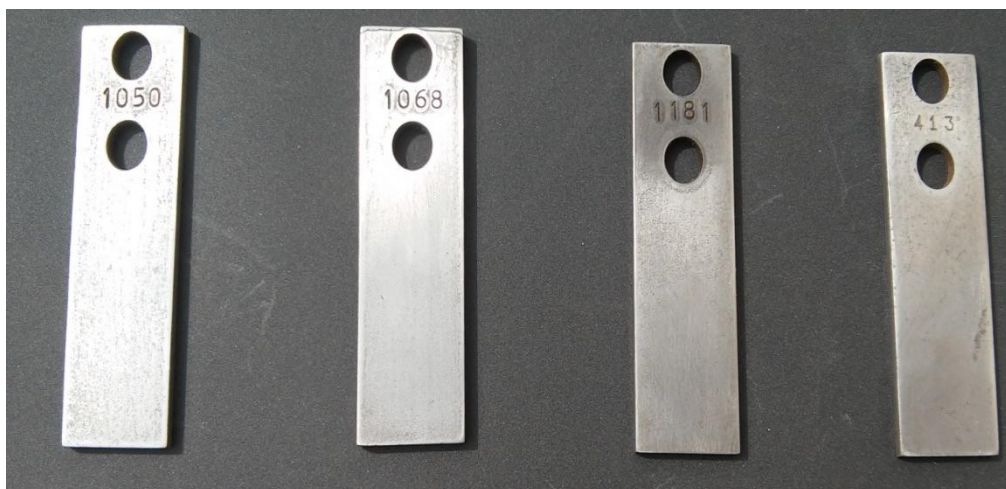
Fig 2.1: Samples as after surface preparation (with mirror finish)
