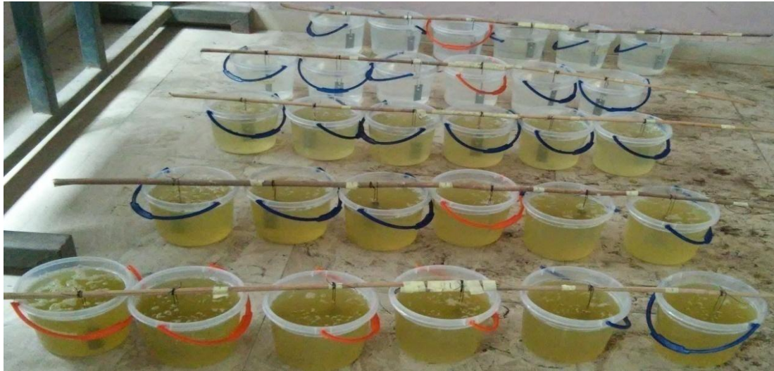
Fig2.3: The flow diagram representing the test inside a solution of HCl with carica papaya leaf extract.
