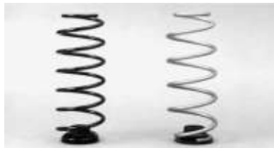
Fig. 8. Rear axle spring of the Lupo FSI (left: steel, right titanium alloy Low Cost Beta [LCB])
