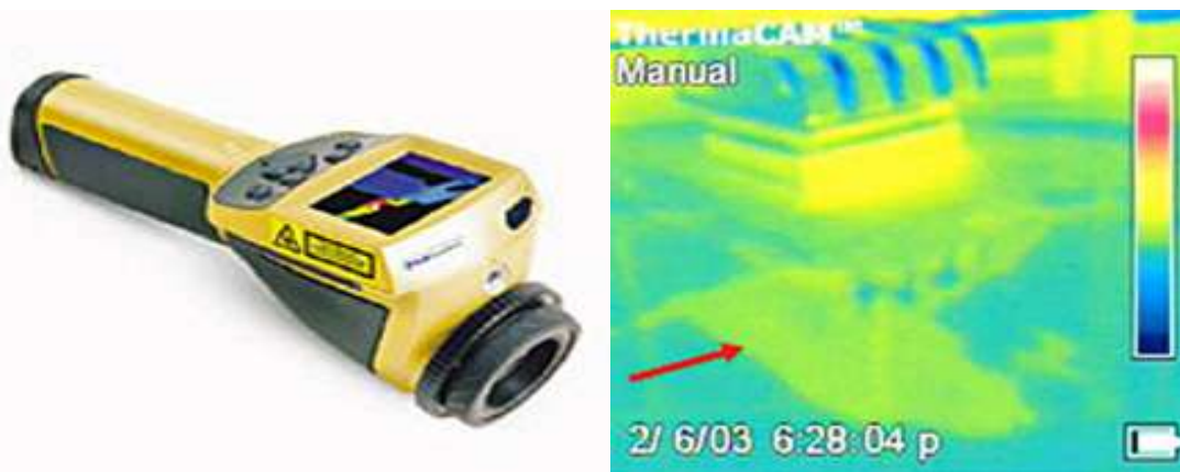
Figure 10. FLIR ThermoCAM ES IR camera and IR photo
