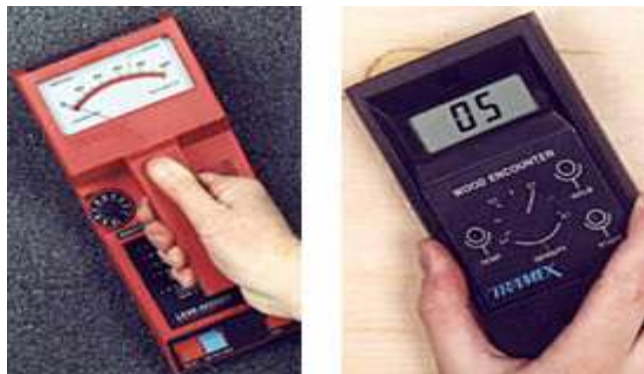
Figure 9. Tramex Capacitance meters
