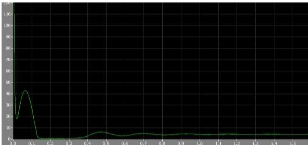
Fig.10. Input current waveform for 470\mu\text{F} and input impedance of 0.1\Omega
