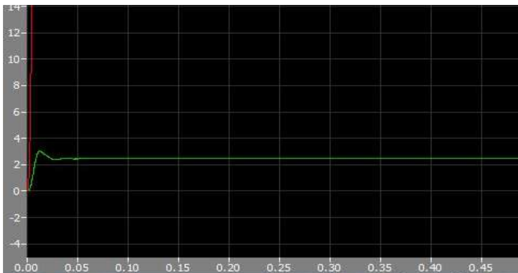
Fig.15. Output current waveform for 470 \mu F and input impedance of 0.4 \Omega
