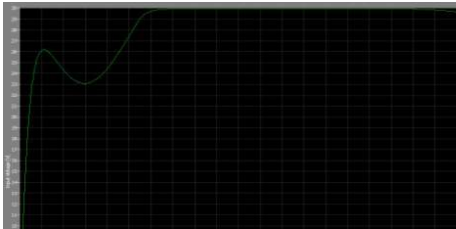
Fig.8. Input Voltage waveform with input capacitance (1000 \mu\text{F} )
