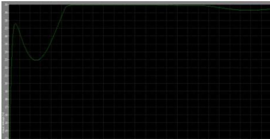
Fig.7. Input Voltage waveform with input capacitance (470 \mu\text{F} )
