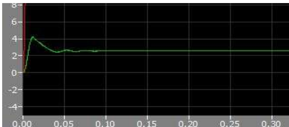
Fig. 13. Output current waveform for 470 \mu F and input impedance of 0.1 \Omega
