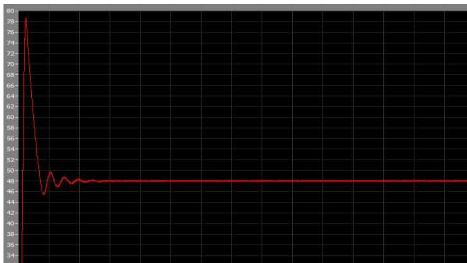
Fig.12. Output voltage waveform for 470 \mu F and input impedance of 0.1 \Omega
