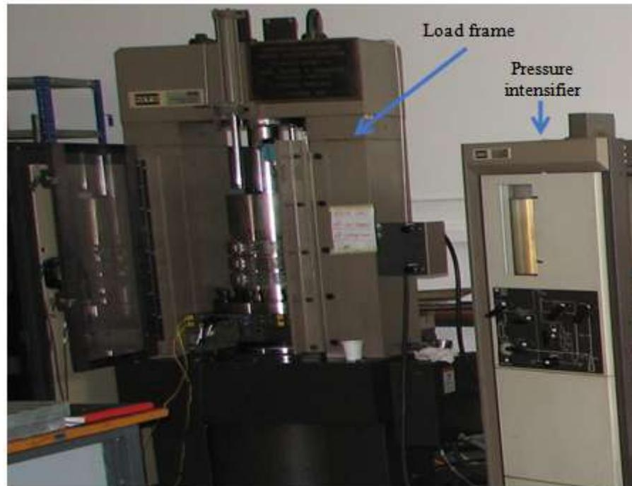
**Figure 4:** Servo-controlled testing machine and pressure intensifier
