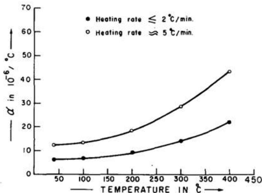
Figure 3: Effect of temperature and heating rate on the coefficient of thermal expansion of granite (Ramana and Sarma, 1980).
