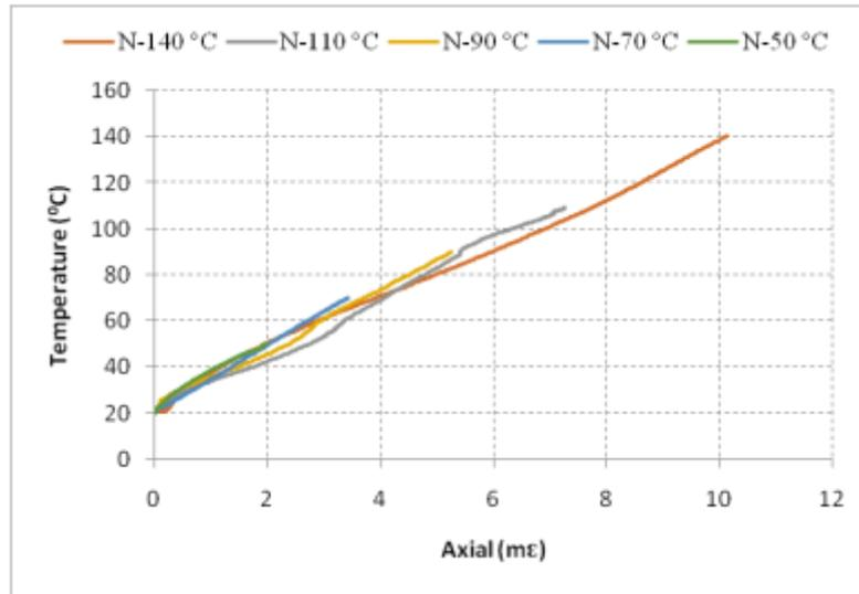
**Figure 7:** Plot of temperature versus axial strain for norite under 10 MPa confinement
