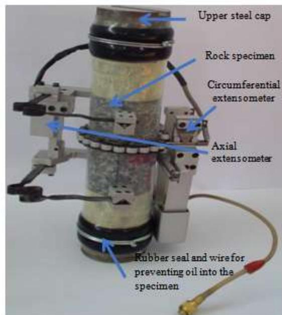
Figure 6: Axial and circumferential extensometers attached to Norite specimen – ready for testing.
