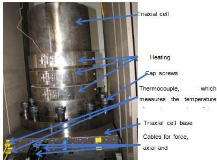
Figure 5: Parts of MTS servo-controlled triaxial cell
