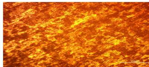
Plate 5: Optical Micrograph of 316 ASS Heat Affected Zone after corrosion (x100)
