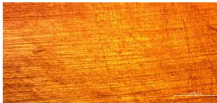
Plate 4: Optical Micrograph of 316 ASS Base Metal after corrosion (x100)
