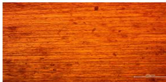
Plate 4: Optical Micrograph of 316 ASS Base Metal after corrosion (x100)
