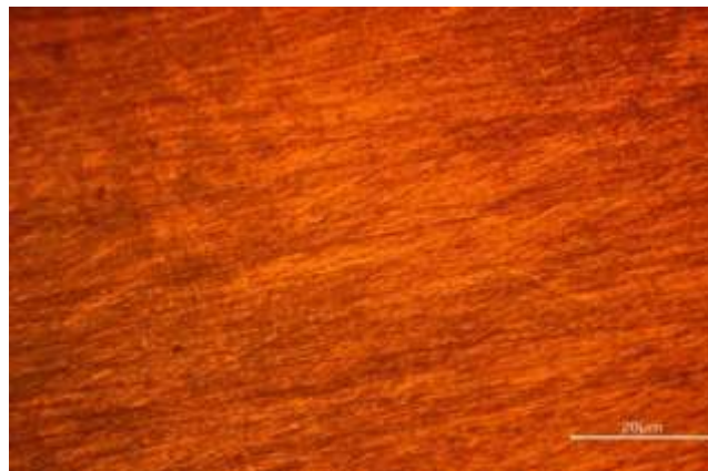
Plate 2: Optical Micrograph of 316 ASS Heat Affected Zone (HAZ) (x100)
