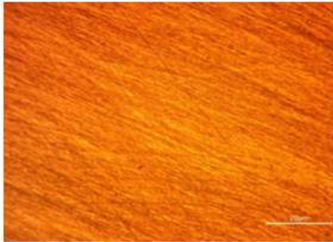
Plate 1: Optical Micrograph of 316 ASS Base Metal (BM) (x100)
